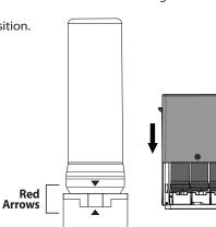
**HELPFUL TIP:** If you find it difficult to screw in the filter, wet the O-ring on the filter housing by holding it under the cold water faucet for a quick second.
